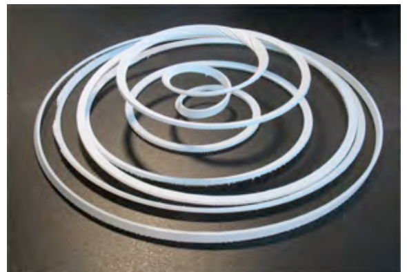
Fig 3.50 Spiral with fully removed support matrix
