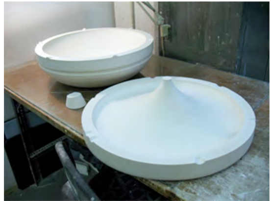
Fig 3.41 2 piece plaster mould
