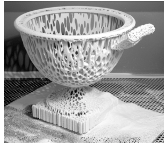
Fig 3.59 The first test piece emerging from the Z Corp RP machine
